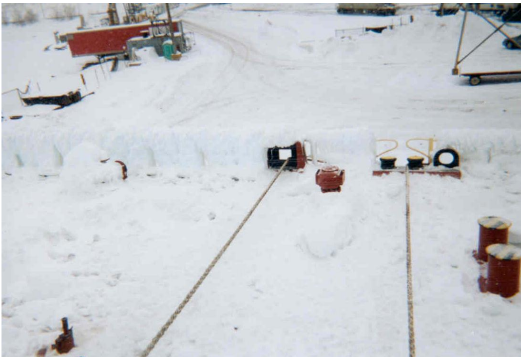
Figures 5.3L– Ship tied up alongside – Railings are walls of ice and decks covered in snow and ice
